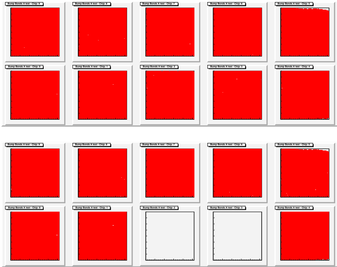
FIG. 13: Bump bond test A results for P_2x5_021_C. The top plot was performed at +20° C and the bottom plot was performed at -15° C.
