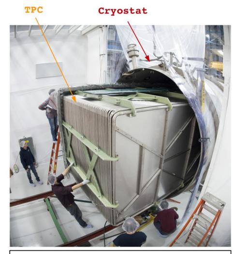
TPC being positioned in cryostat
