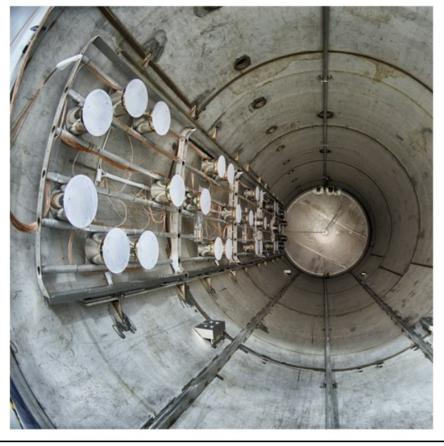
Looking inside cryostat, before TPC inserted
