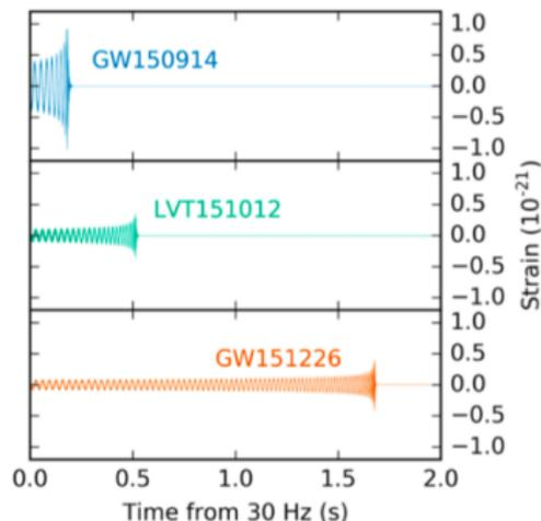
Time evolution of the waveforms after entering LIGO band-pass. From LSC et al. (2016).
