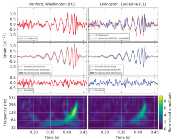
LIGO measures strain,  $\frac{\Delta l}{l}$ . The strain pattern from systems of merging compact objects is oscillatory. The strains from the two detectors were consistent with the time of flight.
