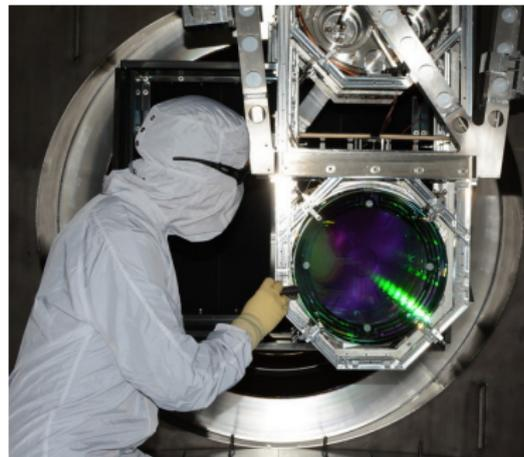
The advanced LIGO test masses are supported on 4 pendulum system. Earthquakes, wind, and trucks are still a problem. This they solve by two LIGO separated by 10ms of light travel and demanding both see the same signal.
