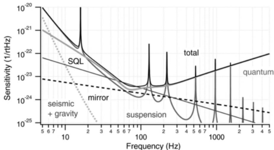
LIGO sensitivity is limited by jitter in the length of the light storage arms. Ground shake is dominant at low frequency jitter. “Quantum” noise is just shot noise in the photons hitting the mirrors— buy a bigger laser or learn about squeezed light. “SQL” is suspension thermal noise and actuator noise- try better coatings. The mirror support is fantastic, see the next slide, but it rings.
