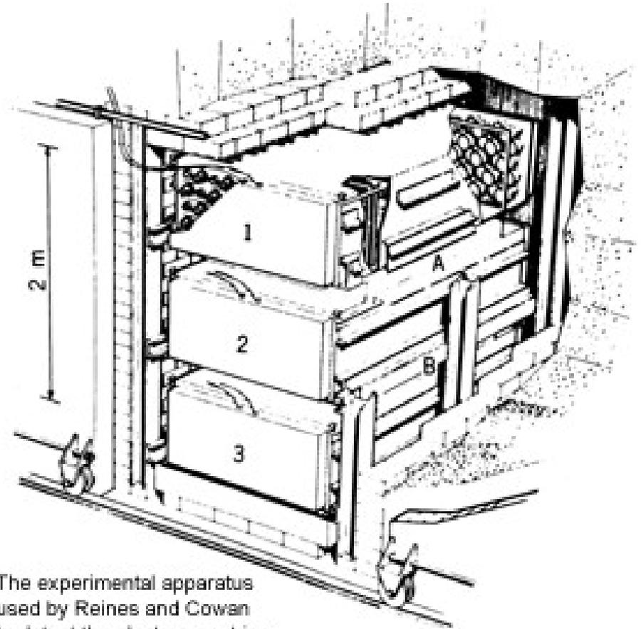
The experimental apparatus used by Reines and Cowan to detect the electron neutrino.
