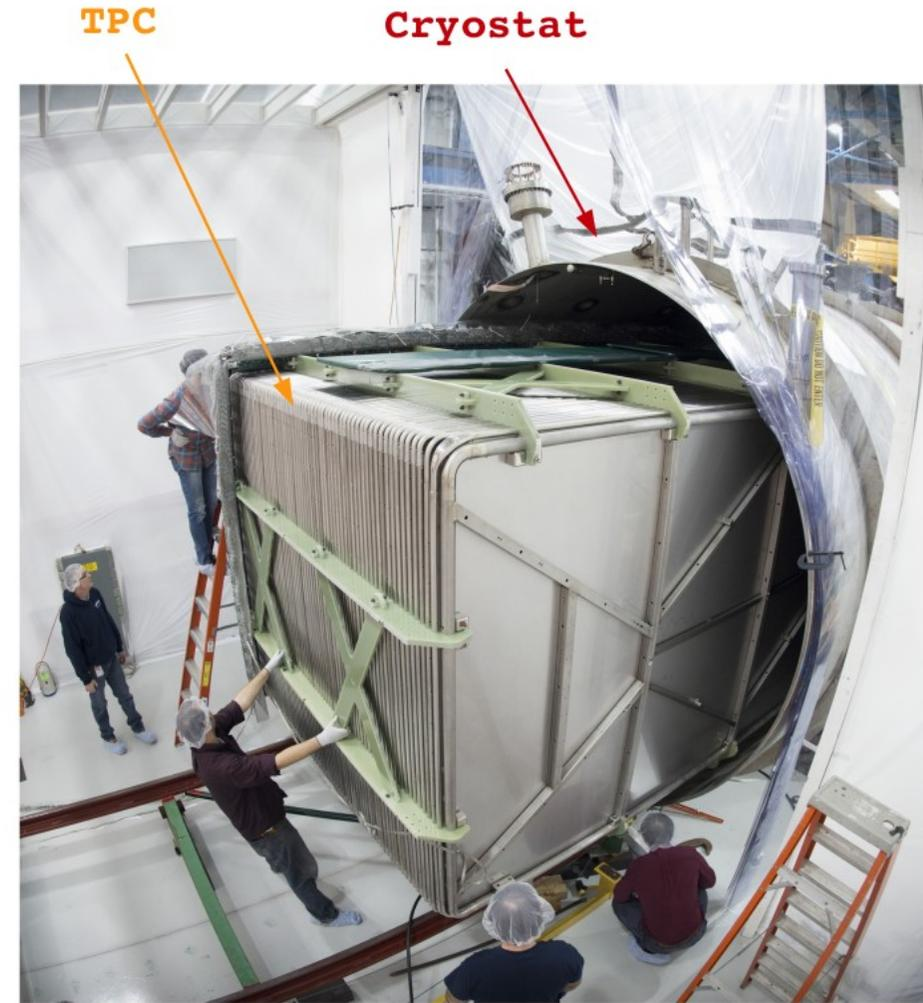
TPC being positioned in cryostat
