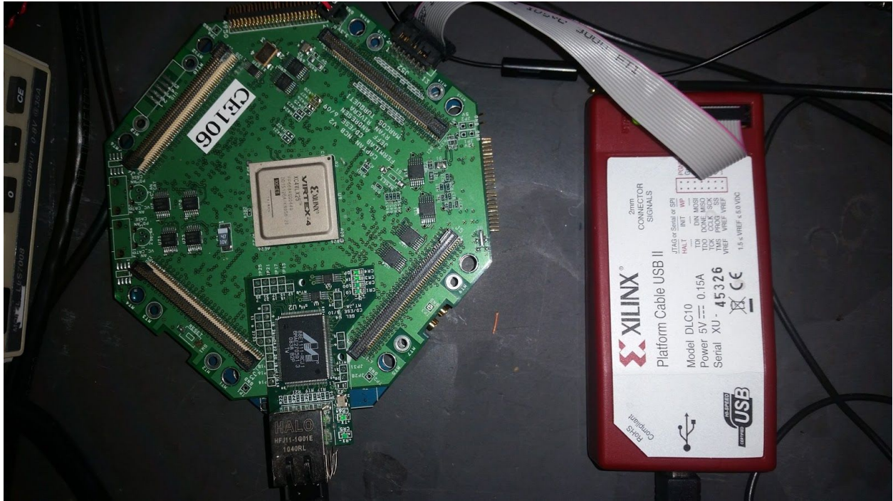
Captan board (left) with ADC (blue mostly hidden by Captan board. You can see a small blue square on the bottom of the image. That's the ADC board. ) and the Xilinx JTag programming cable (red box to the right).
