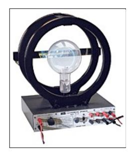
To use the Helmholtz apparatus, turn on the power supplies. Allow the filament of the electron tube to warm up for a minute or so. When the filament is glowing, slowly turn up the accelerating voltage. Then you can adjust the current to the coils to see what happens.
